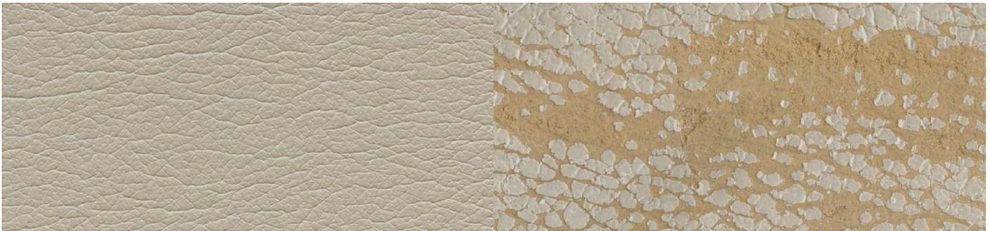
**Note:** The number of weeks of hydrolysis testing has no direct correlation to years of service in the field.
